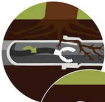
◀ Pipe with ROOT INTRUSION being cleaned with a cable fitted with a root-cutting blade.
